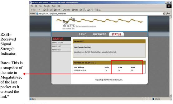
connected. The page will also show the Mode, Rate and RSSI communication information for each connected Client SU.
